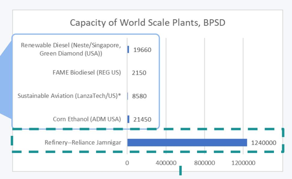
Scale mismatch in state of the art refineries vs next generation, low carbon fuels
