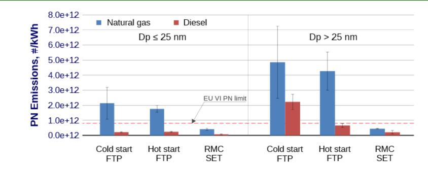
3. Solid PN emissions from a CNG engine and a diesel engine with a DPF for particles below and above 25
